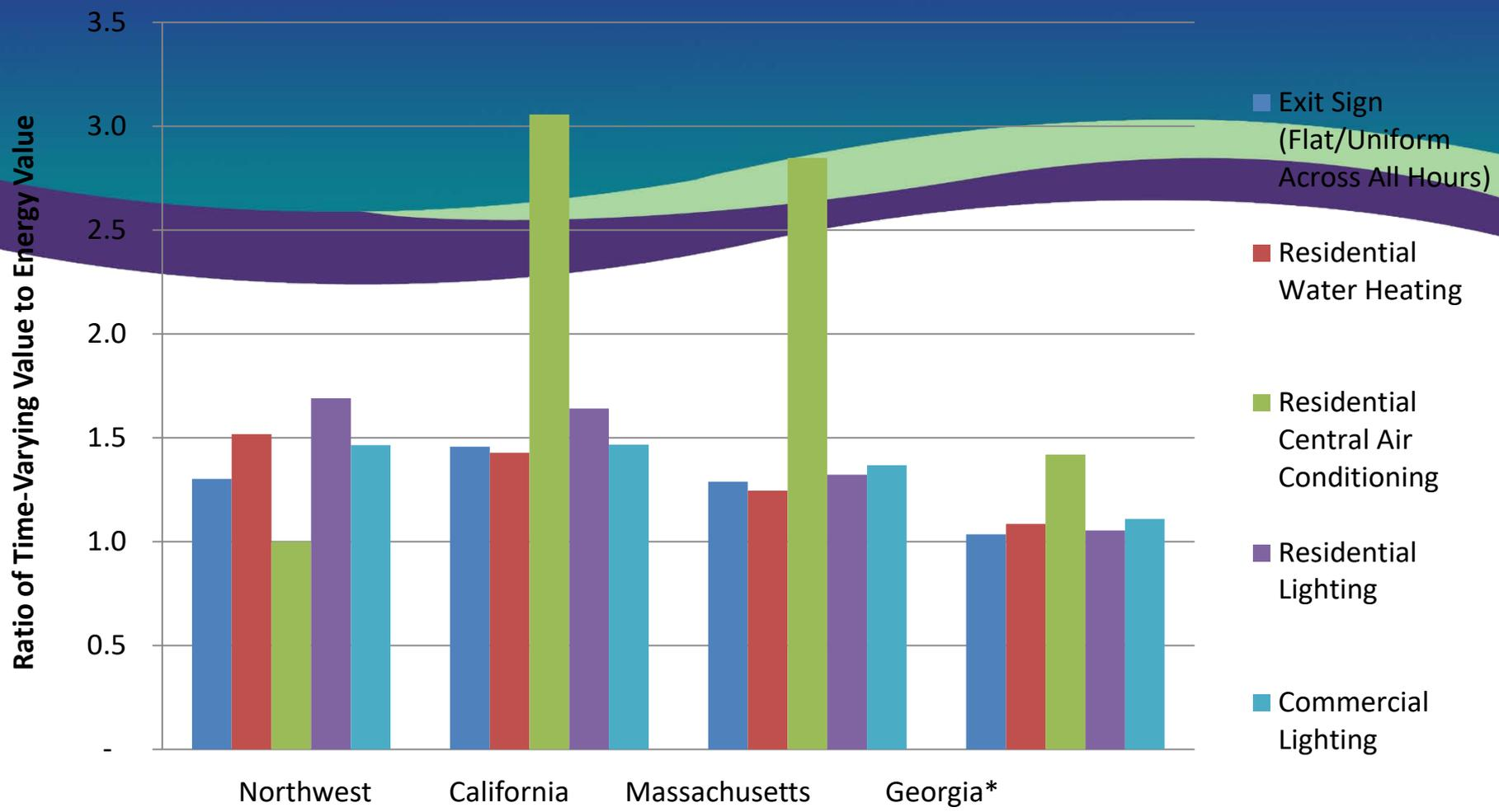
Notes: The flat load shape is an exit sign. Energy value includes: energy, risk, carbon dioxide emissions, avoided RPS and DRIPE, as applicable. Total time-varying value includes all energy values and capacity, transmission, distribution and spinning reserves. Ratios are calculated by dividing total time-varying values by energy-only values.
